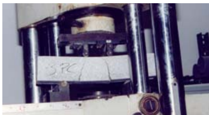
Figure 10. Specimen during bending test.
